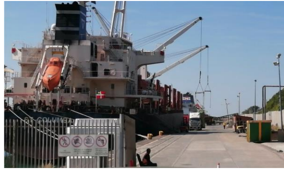
Figure 21: Loading Operation with Ships Gear
